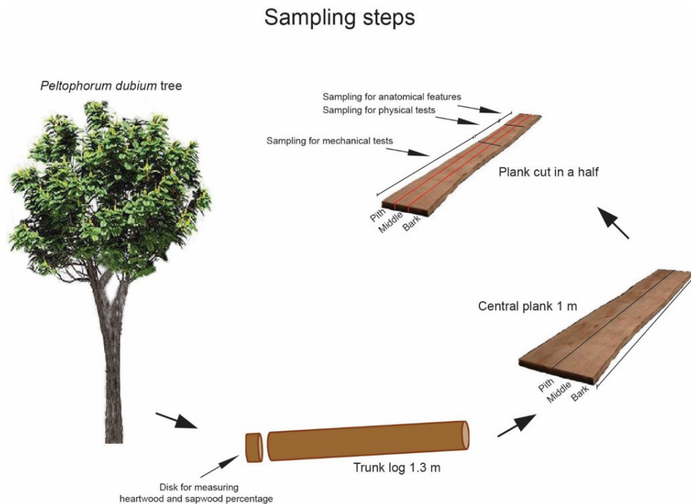
Figure 2. Schematic illustration of sampling for determination of heartwood and sapwood percentage and specimens' origin to determine the physical-mechanical tests and anatomical features.
